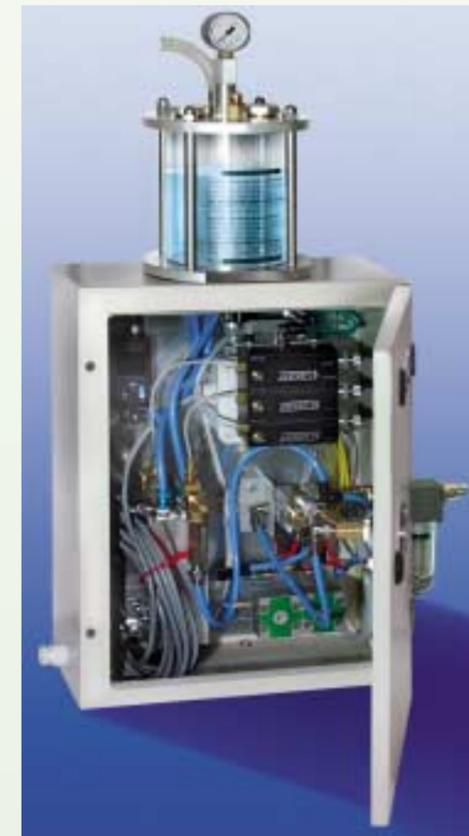
The new developed **micro-lubrication-system** is appropriate for coolant fed tools in CNC-machining centres and CNC-turning lathes.
